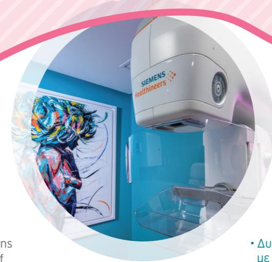
**Mammomat Revelation Mammography System** made by Siemens Healthineers, capable of conducting digital mammograms, tomosynthesis, 2D and 3D reconstructive images, contrast-enhancement mammograms, stereotactic biopsies and tomosynthesis biopsies. It features the innovative PRIME technology which reduces radiation exposure by up to 30% plus the best possible imaging.
